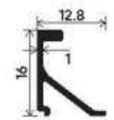
Mosquito Shutter Clip Section Number : V-2514 Weight (kg/mt) : 0.144
