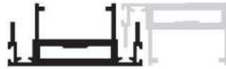
Double Side Interlock Section Number : V-3528 Weight (kg/mt) : 1.150
