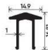
"V" Type Track Rail Cap Section Number : V-3581 Weight (kg/mt) : 0.157
