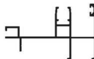
Additional Track Section Number : V-3560 Weight (kg/mt) : 0.956
